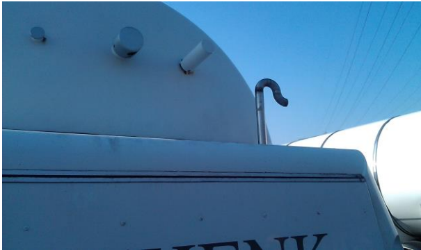
Tanker truck blow-off pipe
