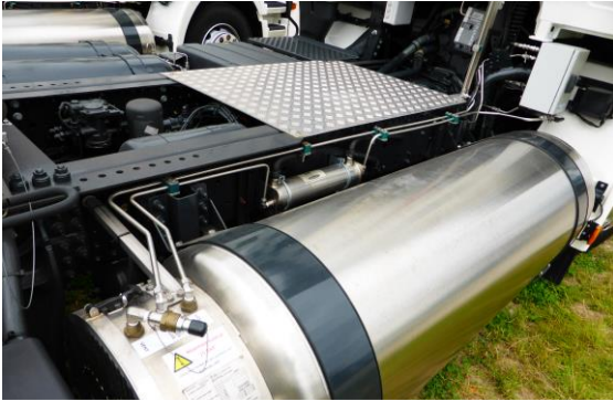
LNG on the side of the truck. There are one or more blow-off valves in the section on the left (under flap and pipes).
